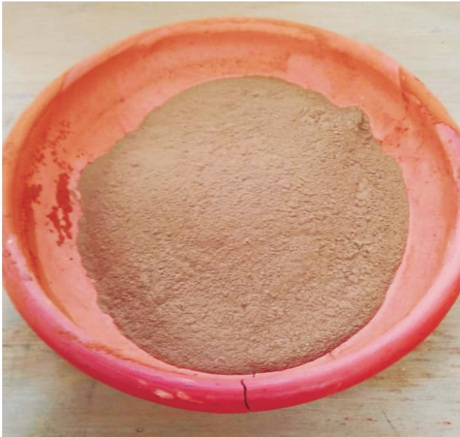
Figure 3. HTK at 600 ° C after two hours of exposure. Source: Authors.
