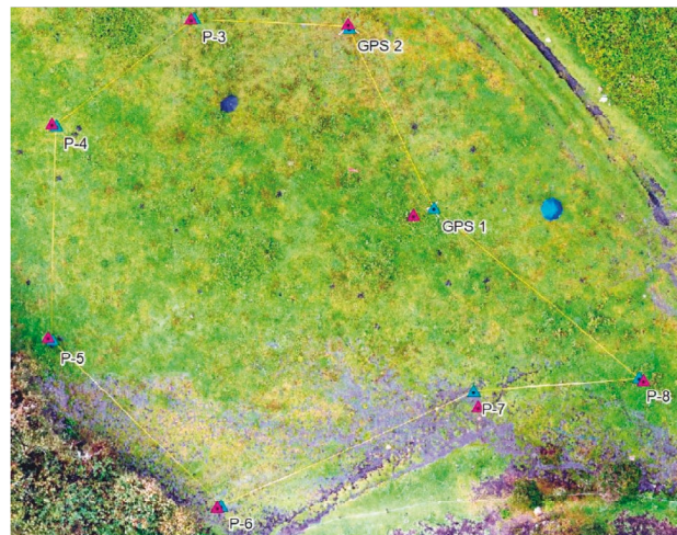
Figure 9 Positional difference between GNSS and Azimuth & Distance with declination correction
